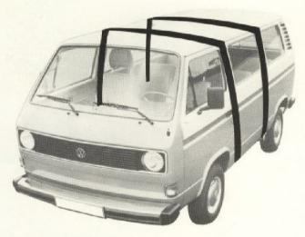
To begin with, there are two strengthening ribs in the roof panel which are welded to vertical pillars; if these are cut or removed the strength of the body shell and the safety of passengers will be impaired.
